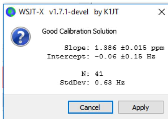
For a quick visual check of the resulting calibration, stay in **FreqCal** mode with the **Measure** option cleared. *WSJT-X* will show the adjusted results directly on the waterfall and the displayed records.
