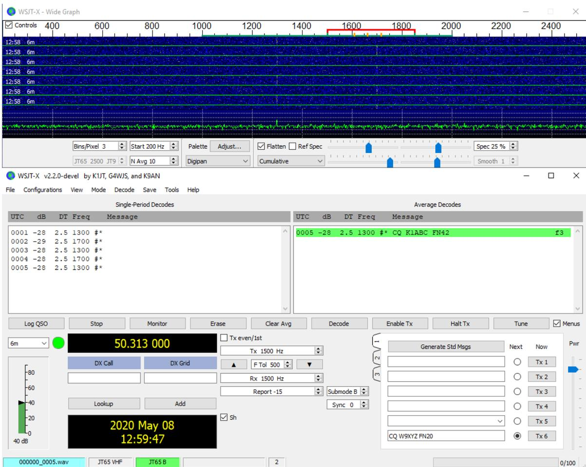
The message **CQ K1ABC FN42** appears in the *Average Decodes* panel, flagged with the **end-of line label f3**. The label means that decoding was accomplished with the Franke-Taylor algorithm, using the average of 3 transmissions.
